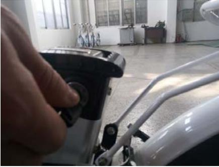
**D.** Turn on the power (turn left the key under the battery box)
