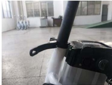
**B.**Put the battery into the battery container beside the seat tube and to the end from lead rail and keep it connect well and stable.
